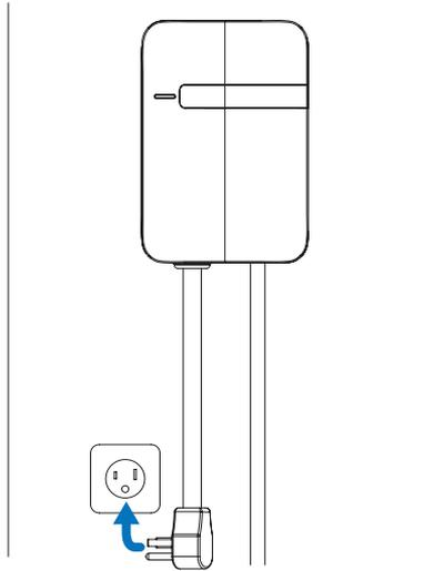
Figure 2-5 Plug in the power cord
