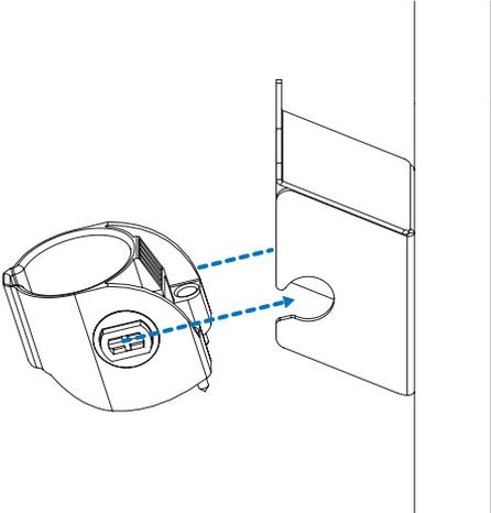
Figure 2-13 Secure the holster
