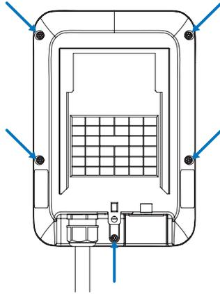
Figure 2-6 Position of five screws on Base Cover
