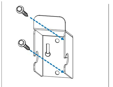
Figure 2-12 Secure the hook
