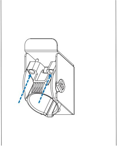
Figure 2-15 Secure the hook
