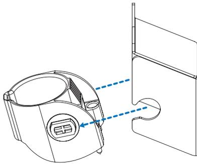
Figure 2-11 Separate the holster
