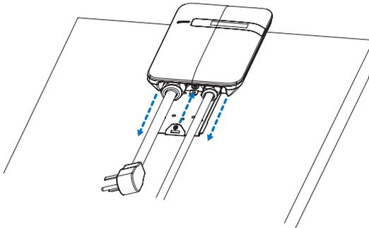
Figure 2-4 Tighten M4 screw
