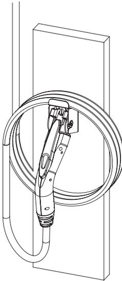
Figure 2-16 Place NC7000 series charging plug.
